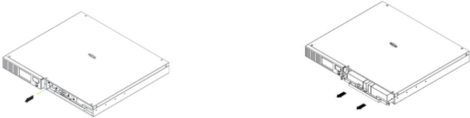
4. Remove the retaining screw of the cable connectors.
