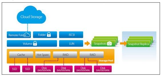
Each layer is designed to cover an aspect of the storage system, and all four layers combined can achieve total protection for your storage system.
