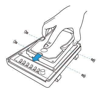
b. For TS-212P and TS-251C: Place the first hard drive in the hard drive cradle and slide it forward to look it into the connector. Place the second hard drive on top of the first hard drive and secure the screws on the slides of both hard drives. Connect the SATA cable and power cable to the connectors as shown in the picture.
