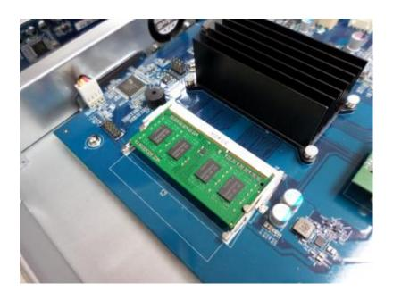
Note: For TS-x53U & TS-451U models, always ensure that a memory module is installed in the primary slot (red box in the below figure,) or the system will fail to start. When installing two memory modules, please ensure that they are the same size and ideally use the same type of RAM for both memory slots. The maximum supported memory is 8GB combined.
