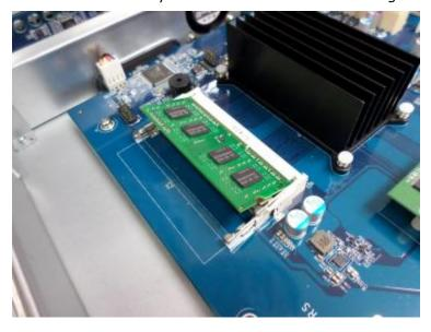
4. Press the memory module down. Make sure the memory module sits in properly with the clips in place.
