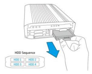
3. Attach the drive to the tray and secure the four screws in the back of the drive tray.
