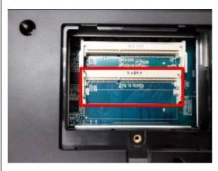
3. Slide the memory module to the slot at a 45-degree angle (approximately) and press
