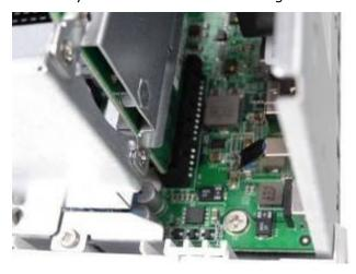
6. Always ensure that a memory module is installed in the Primary slot (red). If not, then the system will fail to start. When installing two memory modules, please ensure that they are the same size and ideally use the same type of RAM for both memory slots. The maximum supported memory is 8GB combined.
