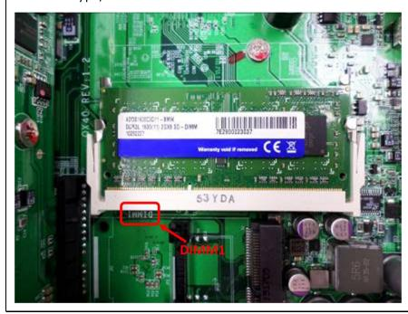
3. Slide the memory module to the slot at a 45-degree angle (approximately) and press the memory module down until it clips into place. Ensure the memory module sits properly with the clips in place.
