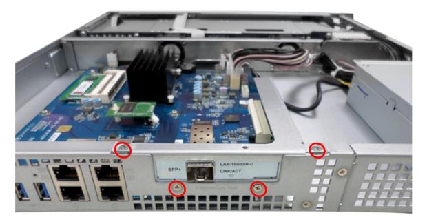
6. Grasp the metal edge of the riser card module. Remove the module gently.
