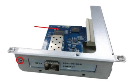
9. Align the notch on the gold edge of the riser card with the notch in the PCIe slot. Insert the riser card module to the PCIe slot until it cannot go any further.
