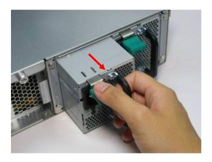
4. Plug in a new power supply to the NAS.
