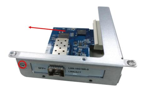
b. For TVS-471U, loose the screw and remove the bracket
