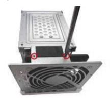
5. Gently remove the hard drive cage from the NAS by lifting it out of its slot.
