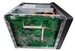
4. Grasp the edge of the memory module. Align the notch on the gold edge of the module with the notch in the memory slot. Slide the memory module to the slot at a 45-degree angle (approximately).
