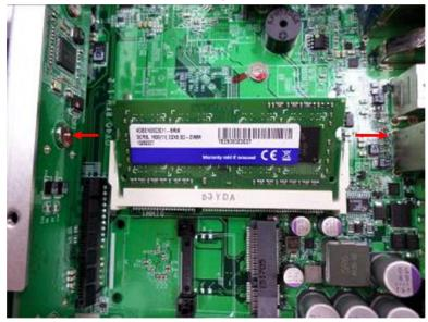
Note: Always ensure that a memory module is installed in the primary slot that is
