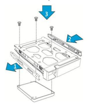
3. Insert the hard drive tray into the Turbo NAS all the way to the bottom and close the case cover.
