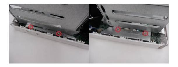
4. If it is a 4-bay NAS, you will also need to remove two screws on the top of the hard drive cage.
