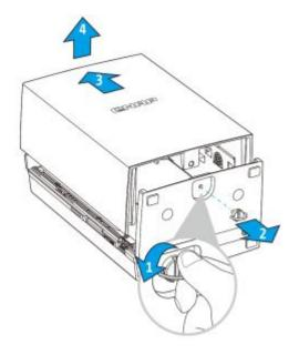
2. Put the hard drive in the hard drive cradle and slide it forwards to lock it into the SATA connector. Clip in both brackets, slide the bracket into the hole in point 2 before pressing the bracket towards the HDD (for the TAS-268, repeat the same step for the second drive.)
