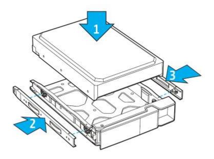
b. For 2.5" HDDs/SSDs, only remove the bracket next to the 2.5" screw holes (they are marked on the bottom of the tray.) Secure the three screws in the back of the hard drive tray.
