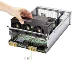
Fan modules can also be easily replaced.
